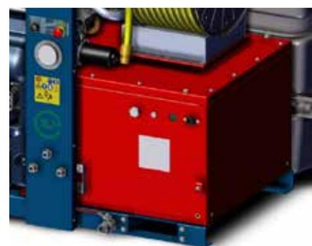
17.6 kW lithium batteries. Autonomy 3300 lt.
