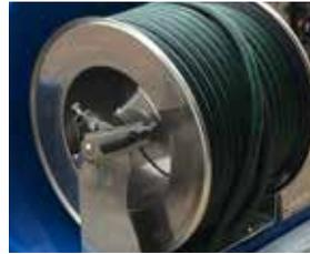
New design with ABS cover and key-lock system
